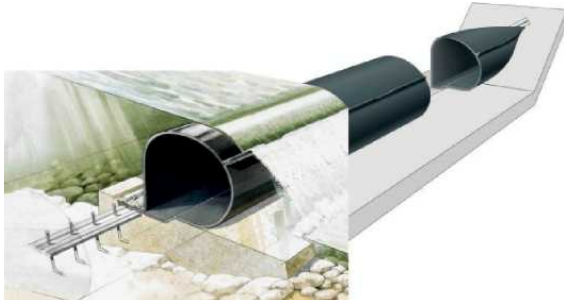
Fig. 1. Rubber dam axonometric section. This figure shows how rubber body is secured to a concrete foundation by its anchor line.
