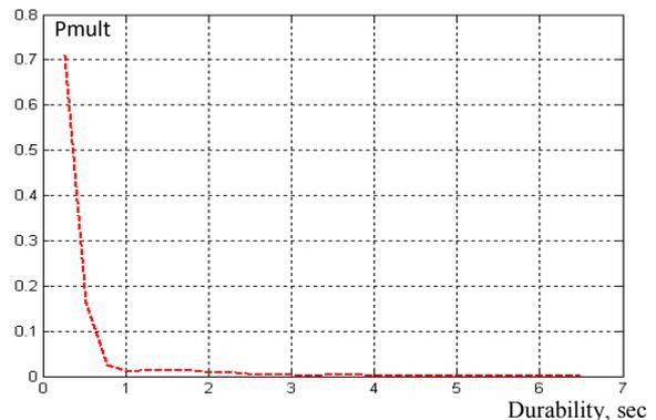
Fig. 2. Distribution of durability of abnormal measurement results
