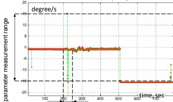
Fig. 1. Graphic representation of TMI with grouped abnormal outliers (angular rate sensor of a flight vehicle)
